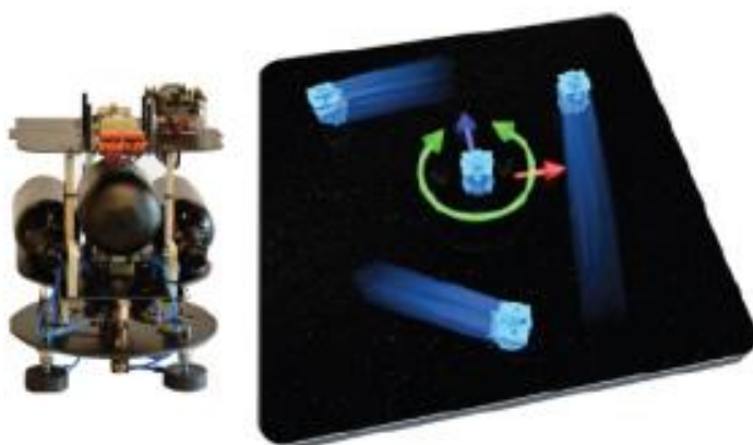
Fig. 2: Beacon based positioning will be initially tested on the S.M.S. - Satellite Manoeuvring Simulator (right). Here an air cushion based S.M.S.-vehicle (left) can move in an 2D-setup between the beacons.
