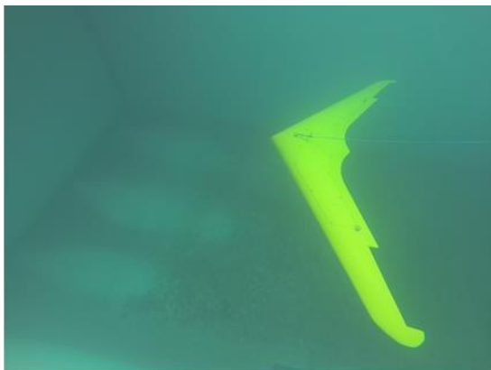
Figure 1: The underwater glider MOTH in the 5 m deep test basin of MARUM
