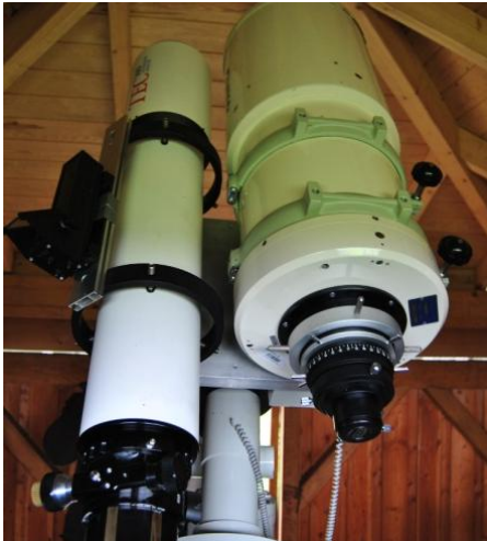
Fig. 1: Telescopes mounted at Liebenhof Observatory: TEC 140 Apo Refractor (left, 140 mm aperture, 980 mm focal length, 0,81° field of view) and Baker Ritchey Chrétien (right, 250 mm aperture, 1268 mm focal length, 0,62° field of view).
