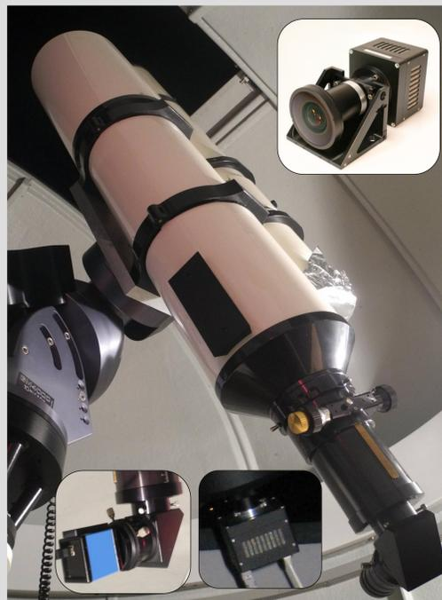
Fig. 1: Observing System: TMB-Refractor and our two cameras (left: DFK 21AU04, right and top: SPOSH camera with and without fisheye lens).
